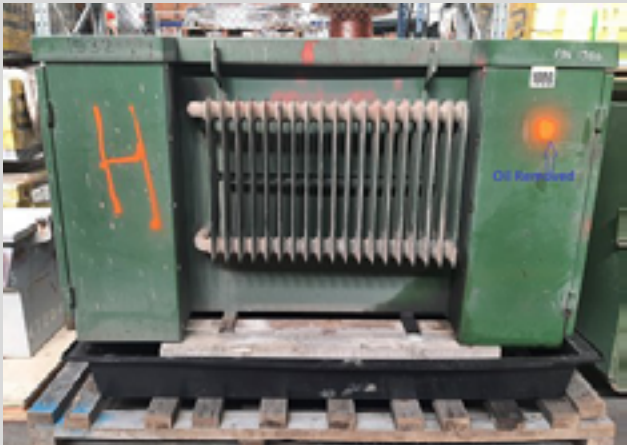
Orange dot indicates oil has been removed from the retired Vector asset by Scope Oil and will be recycled
